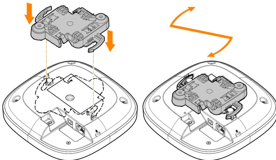
4. Hold the access point next to the ceiling rail with the mounting tabs of the mount bracket at approximately a 30-degree angle to the ceiling rail. Make sure that any cable slack is above the ceiling tile.
